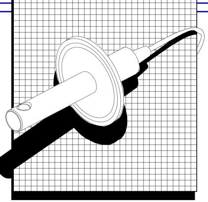
The CS10, CS51 sensors are welded to blind flanges of customer specified size, and can then be inserted into standard tee fittings in sanitary systems using Ladish or Tri-Clover fittings.
